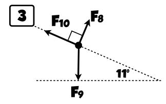
The body is moving up the incline at a constant velocity.
